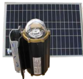
Civil aviation lamp 10 cd complete SET, including 30 m cable, 20watt pv, battery, protection box. Suitable for 130mm or 152mm tubular mast. Code: 08.02.005.SET
