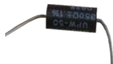
Resistance, high precision 2000 Ohm (to connect PT100 to Stylitis 101 data logger) Code: 25.18.00.004
