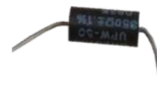
Resistance, high precision 350 Ohm (to connect PT100 to Stylitis 41 data logger) Code: 25.18.00.001
